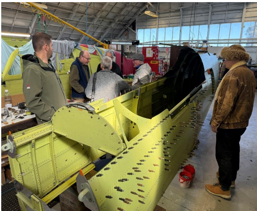
Cockpit area of P40 under construction. The big Allison engine will be at the front of this fuselage.
