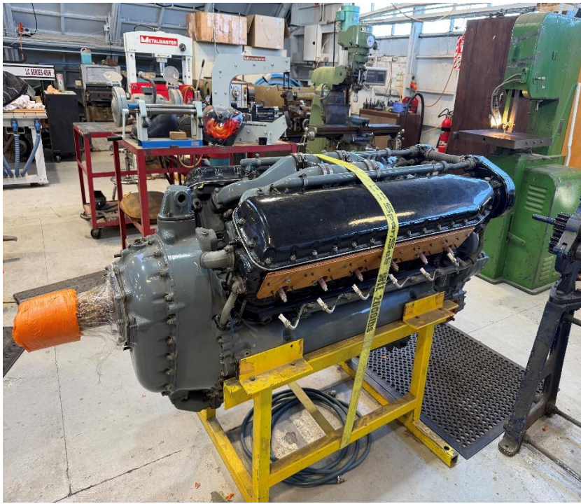
Allison 1000 hp engine for the Curtiss P40
